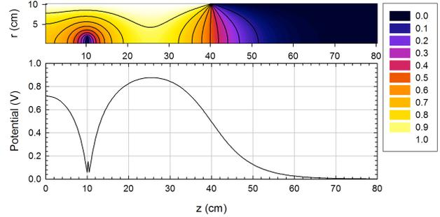
Figure 2: Poisson's equation is solved numerically for the 40-cm-long end electrode at unit voltage, the 0 V deceleration grid at  $z = 10$  cm, and the first 40 cm of 2-m-long main confinement electrodes at 0 V (top –  $r - z$  color contour plot). The presence of the deceleration grid causes the axial-trapping barrier height to be only 87% of the applied voltage (bottom – potential along  $r = 0$ ).
