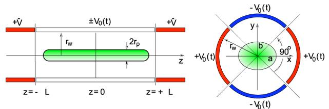
Figure 1: The PTSX device consists of three cylindrical electrodes with radius  $r_w = 0.1$  m, each divided into four  $90^\circ$  sectors. An oscillating voltage  $\pm V_0(t)$  confines the charge bunch in the transverse plane to a radius  $r_p$ . Static voltages  $+\hat{V}$  on the end electrodes confine the ions axially within a length  $2L = 2$  m.
