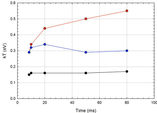
Figure 4: For a plasma that experiences no evaporative cooling,  $kT_{\perp} = 0.17$  eV (black), but  $kT_{\perp} = 0.30$  eV for a plasma where evaporative cooling occurs between  $t = 7$  ms and 10 ms (blue). If the cooling is applied permanently at  $t = 7$  ms, then  $kT_{\perp}$  continues to grow with time (red).
