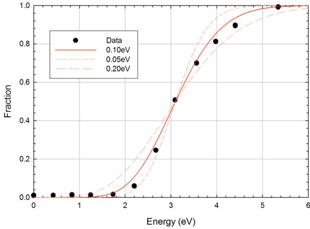
Figure 3: The measured on-axis charge that remains trapped (black dots) drops to zero as the axial-trapping barrier is reduced to zero. The rate of change in the on-axis charge is consistent with an axial temperature of 0.1 eV when the axial distribution is assumed to be a drifting Maxwellian with a mean velocity corresponding to 3.1 eV (solid red line).
