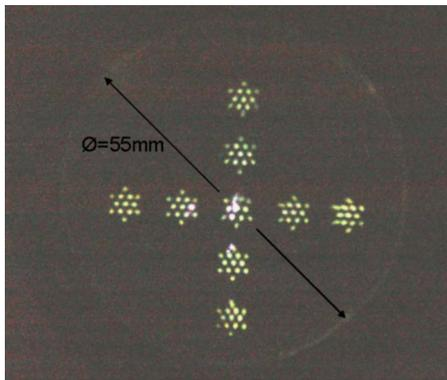
FIG. 6. (Color online) Photograph of the scintillator plate luminescence. Extraction voltage  $U=13.6$  kV.
