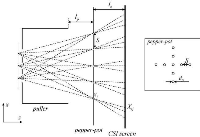
FIG. 5. Scheme of experimental beam emittance measurements by the pepper-pot method (cross section at  $y=0$ ). The small graphical insert on the right corresponds to pepper-pot design.
