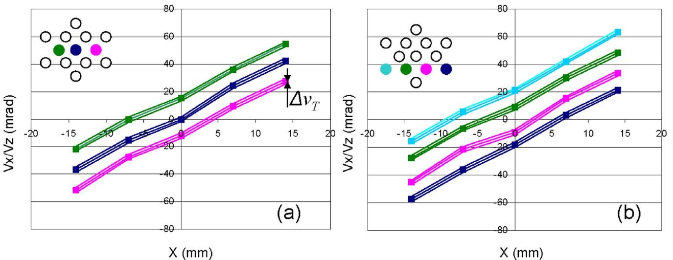
FIG. 7. (Color online) The  $x - V_x/V_z$  beamlet phase portraits reconstructed from Figs. 5 and 6. (a) Phase portraits of the three central beamlets (see the corresponding small graphical insert) and (b) phase portraits of the four beamlets of the first lower row (see the corresponding small graphical insert).
