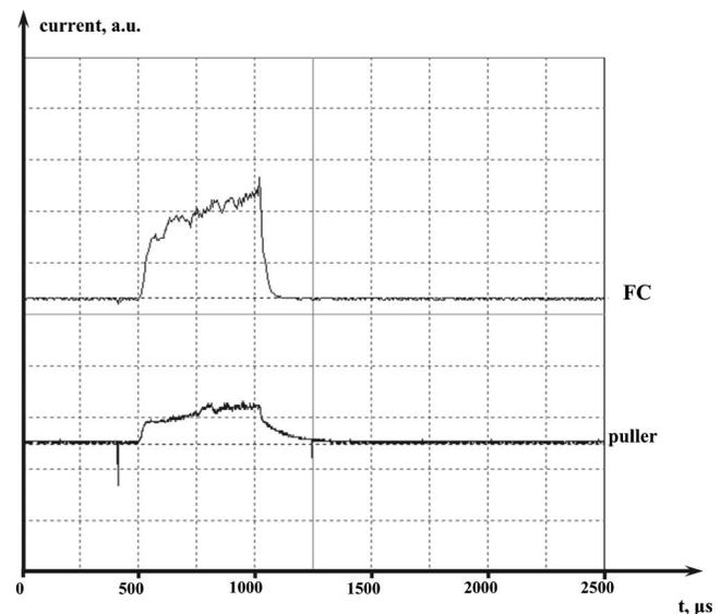
FIG. 4. Oscillograms of the current to the Faraday cylinder (upper trace) and to the puller (lower trace).
