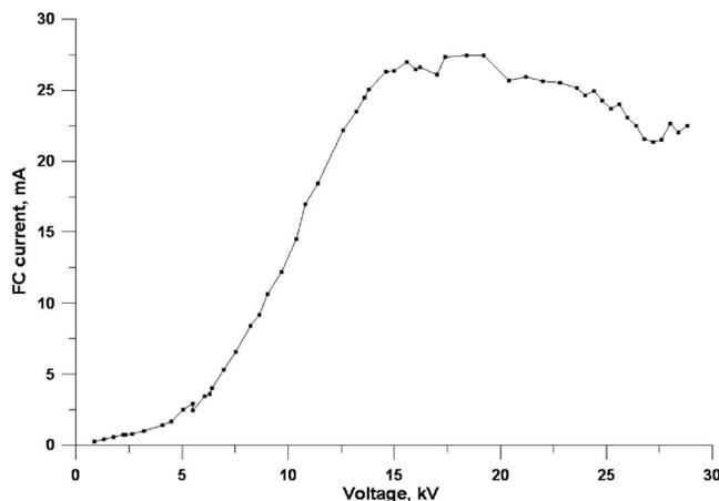
FIG. 2. Extracted ion beam current averaged over 500  $\mu$ s vs extraction voltage.
