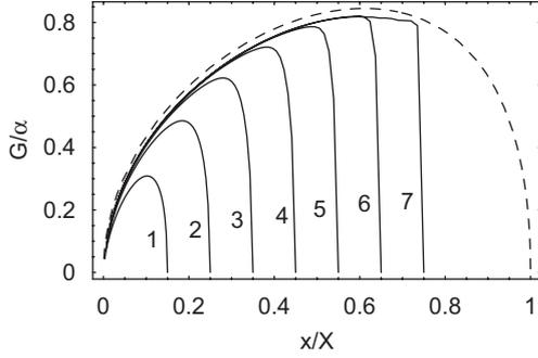
Fig. 2. The normalized instability gain function  $G(x, t)/\alpha$  is plotted as a function of distance  $x/X_f$  at different times  $t/T_f = 0.15$  (1), 0.25 (2), 0.35 (3), 0.45 (4), 0.55 (5), 0.65 (6), and 0.75 (7) obtained numerically (solid curve) and compared with the analytical result in Eq. (33) (dashed curve).
