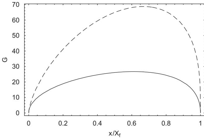
Fig. 3. Comparison of the instability gain as a function of  $x/X_f$  for a beam with velocity tilt (solid curve) and without velocity tilt (dashed curve) for  $\delta_0 = (\omega_{pb}^0/\omega_{pe})^2 = 10^{-3}$  and  $\alpha^2 = (\omega_{pb}^0 T_f)^2 = 1000$ .
