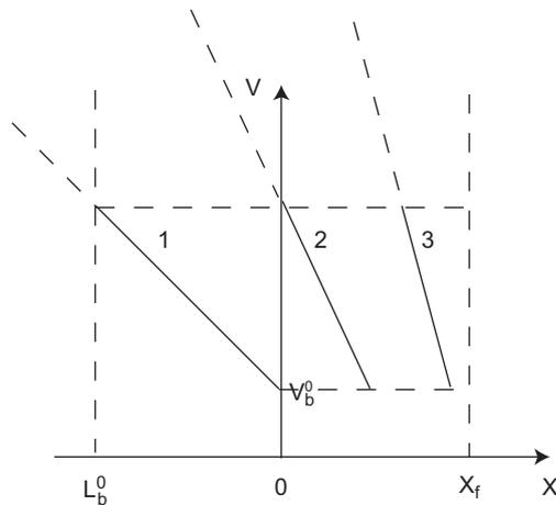
Fig. 1. Plot of the ion beam phase space at different times during the compression (lines 1, 2, and 3). Line 1 corresponds to  $t = 0$ .
