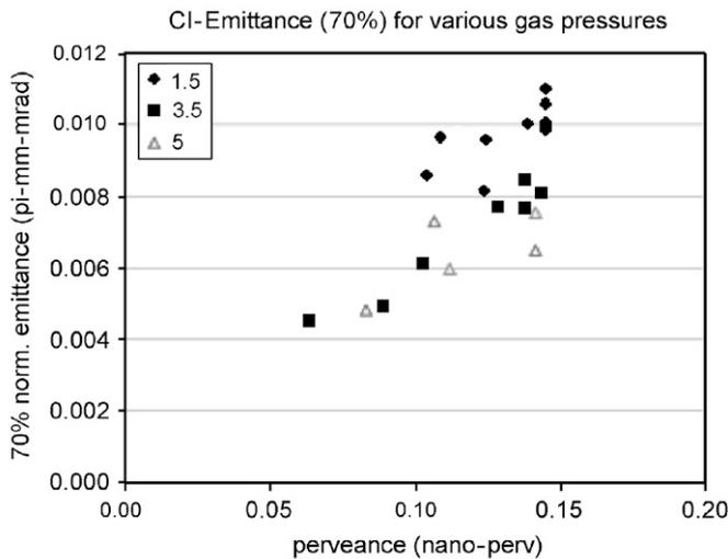
Fig. 3. Normalized  $\text{Cl}^-$  emittance at different source pressures (in mTorr) as a function of perveance [10]. Used with permission from L.R. Grisham, Rev. Sci. Instrum. 77, 03A501 (2006). Copyright 2006, American Institute of Physics.
