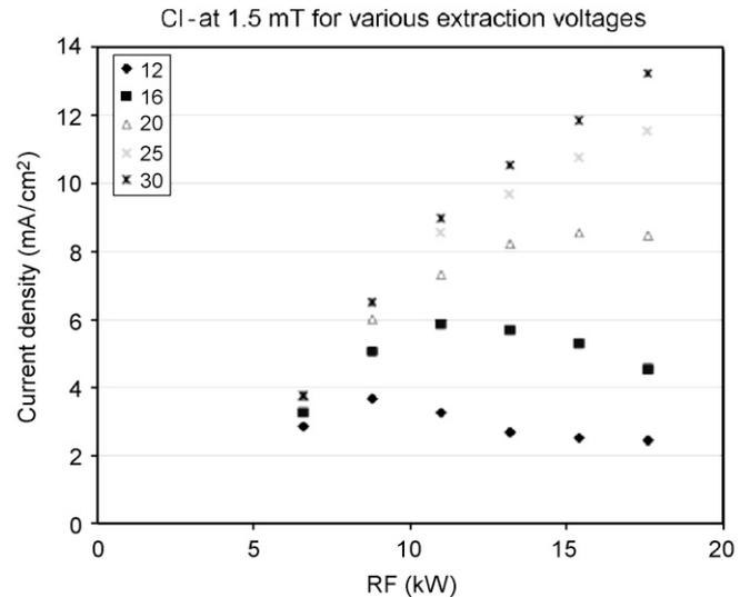
Fig. 2. Faraday cup measurement of the  $\text{Cl}^-$  beam density extracted at various voltages (in kV) as a function of RF plasma drive, at a source pressure of 1.5 mTorr [10]. Used with permission from L.R. Grisham, Rev. of Sci. Instrum. 77, 03A501 (2006). Copyright 2006, American Institute of Physics.
