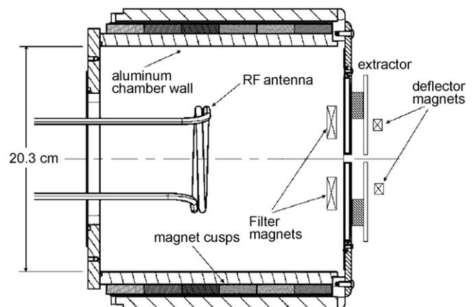
Fig. 1. Schematic of the ion source built for the second experiment comparing negative and positive chlorine with argon. As in other "volume production"  $H^-$  sources, the filter magnets shield the extractor region plasma from high-energy electrons in the driver plasma where the RF antenna resides [10]. Used with permission from L.R. Grisham, Rev. of Sci. Instrum. 77, 03A501 (2006). Copyright 2006, American Institute of Physics.
