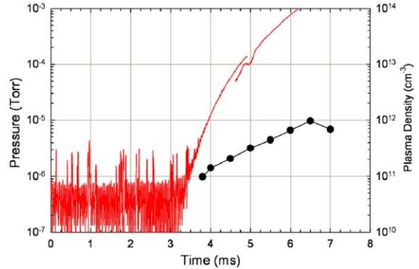
Fig. 1. Time evolution of neutral gas pressure and plasma electron density (solid circles) in the pulsed plasma source.
