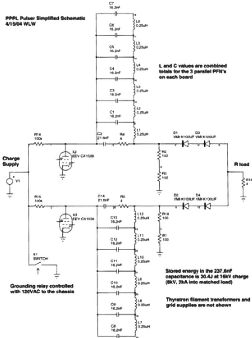
Fig. 3. Schematic of the pulsed power supply.
