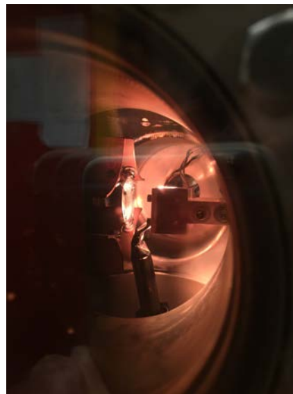
(c) Barium ion source in operation. The assembly includes an iridium plate(right), an oven(center), an extraction grid and four copper plates(left).
