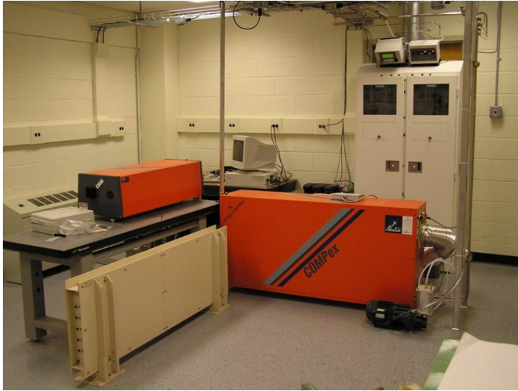
Figure 5.16: Laser system. The small laser on the top a counter is the dye laser. The giant laser on the floor is the excimer laser.
