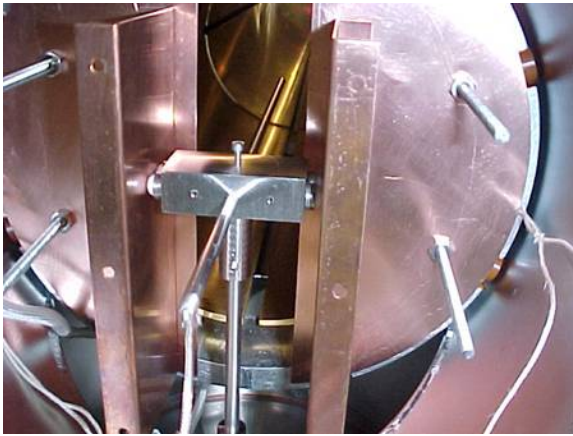
(b) The charge collector is guided in the horizontal direction by a pair of copper plates attached to a slotted copper disk at the end of the PTSX device. (c) The 5 mm diameter head of a copper nail serves as the collection plate.
