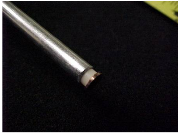
(b) The charge collector is guided in the horizontal direction by a pair of copper plates attached to a slotted copper disk at the end of the PTSX device. (c) The 5 mm diameter head of a copper nail serves as the collection plate.
