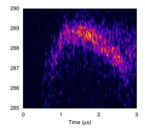
**Fig. 5.** Streak camera image of the longitudinal phase space of the uncompressed beam near the beginning of the pulse.
