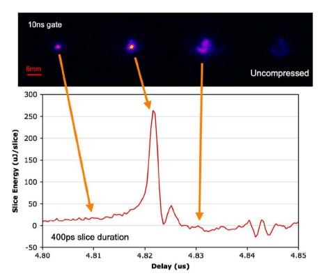
Fig. 7. Time-dependent transverse beam distributions demonstrating the simultaneous transverse focusing at the time of peak compression. The FWHM of the peak is  $\approx$  2.5 ns.
