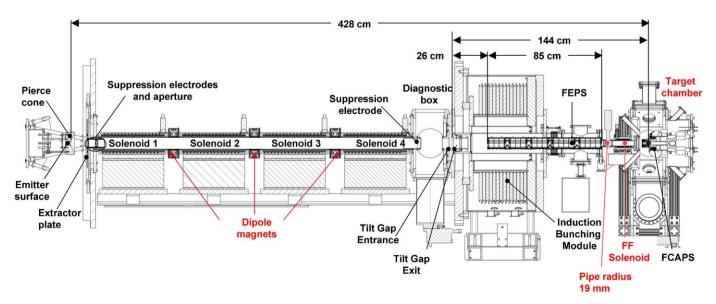
Fig. 1. Elevation view of the Neutralized Drift Compression Experiment.
