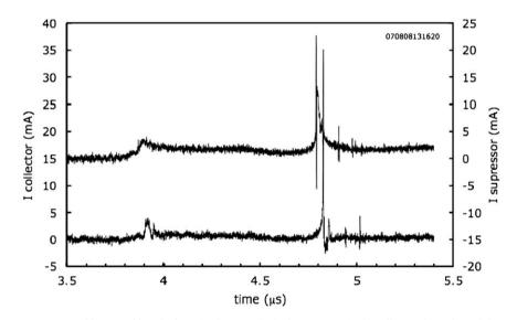
**Fig. 3.** Faraday cup response to uncompressed beam and bunched portion ( $t \approx 4.8 \,\mu$ s). The bottom trace is the collector electrode, and the top trace is the suppressor hole plate.
