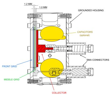
Fig. 2. Fast Faraday cup schematic.
