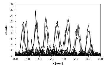
**Fig. 4.** Beam image profiles as a function of focal plane position and deflection plate voltages. The incident beam energy was 289 keV, and the deflection plate voltages were scanned in 50-V steps around 14.5 kV (three shots at each step are shown), corresponding to beam energy variations of 1-keV steps.
