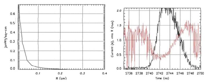
**Fig. 9.** LSP simulations predict a peak energy deposition of 0.69 J/cm<sup>2</sup> at the focal plane (left). In the right plot, the predicted peak current (black) is 2.1 A, with a minimum radius of 0.4 mm (red). The high-frequency oscillations are due to numerical noise (for interpretation of the references to colour in this figure legend, the reader is referred to the web version of this article).
