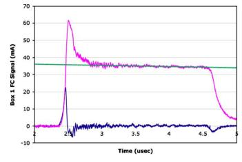
**Fig. 6.** Diagnostic box Faraday cup beam current measurements: the collector plate signal (top), the suppressor grid signal (bottom), and a linear fit to the collector signal flattop.
