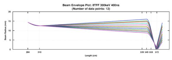
**Fig. 8.** The calculation is initialized at z = 284 cm, at the exit of the IBM gap. The envelope slices are calculated assuming full space-charge contribution, until the entrance to the FEPS at z = 310 cm. The beam propagates assuming full neutralization through the final focusing solenoid (549 < z < 559 cm) to the focal plane (z = 572 cm).
