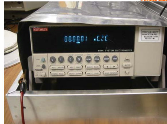
Low level charge measurement (~1 fC)
