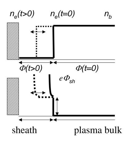
Schematic of a sheath. The negatively charged electrode pushes electrons away by different distances depending on the strength of the electric field at the electrode. Shown are the density and potential profiles at two different times. The solid line shows the maximum sheath expansion.
