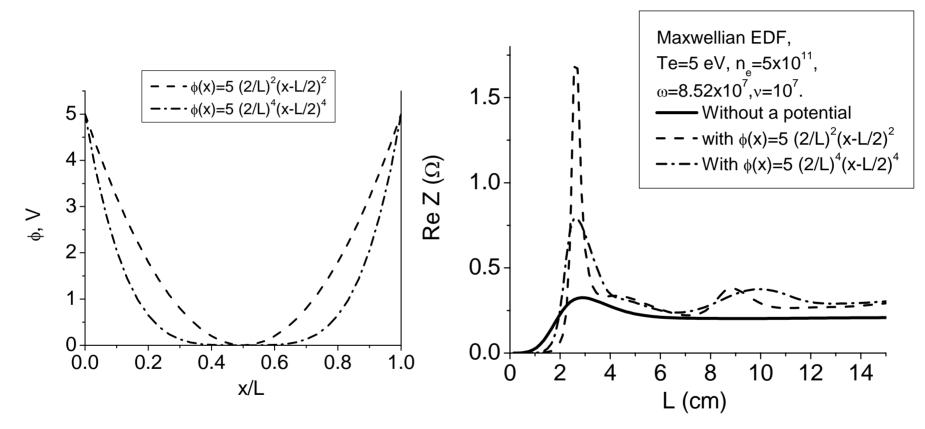
Surface impedance for different plasma profiles.
