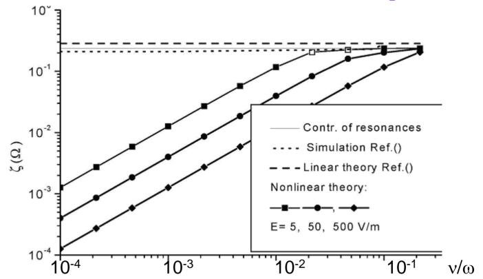
The real part of surface impedance in ohm. The plasma parameters are n=10<sup>11</sup> cm<sup>-3</sup>, T<sub>e</sub>=5ev, l=4cm.
