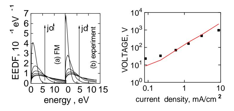
He, p=0.1 torr, ω=13.56 MHz, L=6.7 cm. Experimental data - filled squares, the FM results solid line j=0.085, 0.22, 0.58, 1.3, 6.0, 8.8ma/cm<sup>2</sup>.
