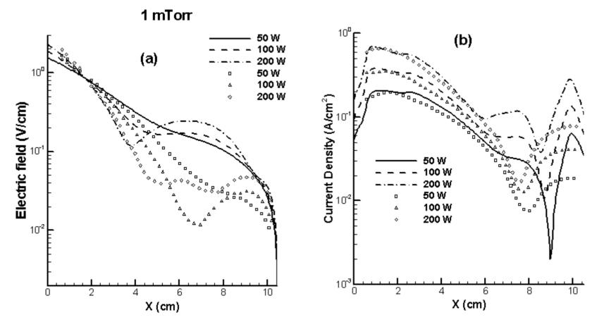
Comparison between experimental data [V. A. Godyak and R. B. Piejak, *J. Appl. Phys.* **82**, 5944 (1997).] and simulation predictions using a non-local model (a) RF electric field and (b) the current density profiles for a argon pressure of 1 mTorr.
